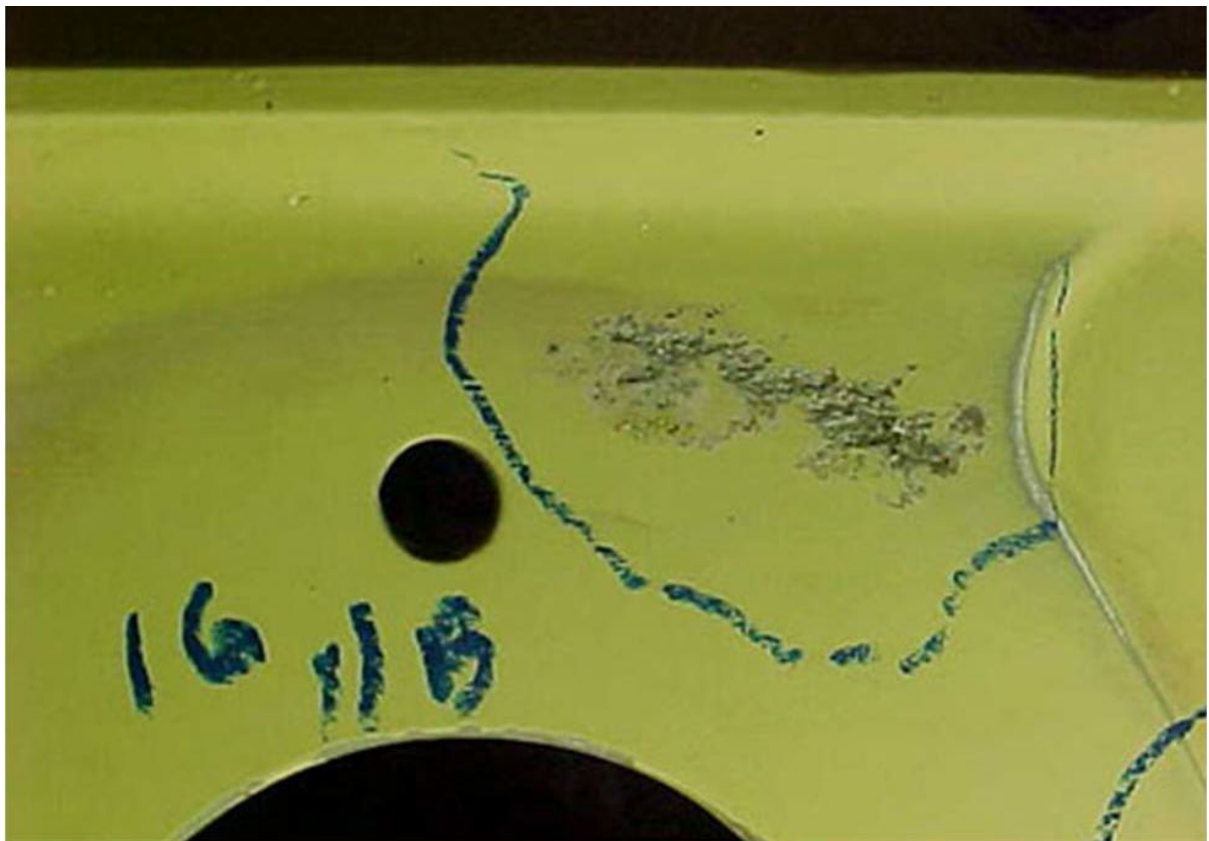
Figure 2: MIC on Aircraft Fuel Tank Walls [10]
